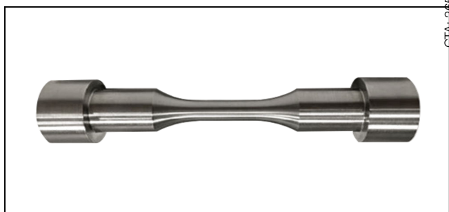
Round specimen with button head for creep fatigue test
