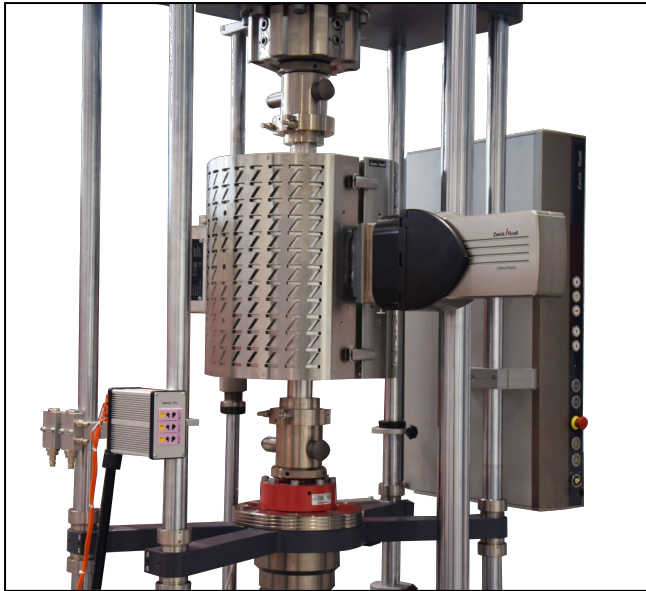
videoXtens 1-32 HP/TZ with closed furnace
