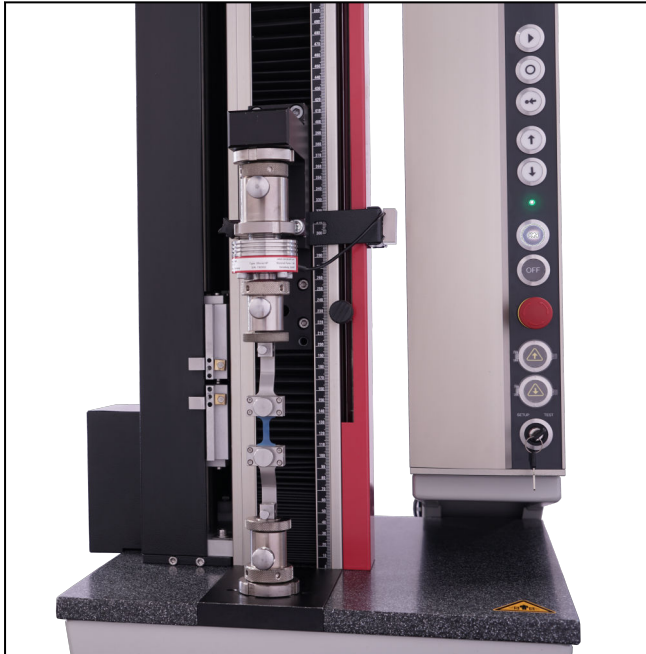
Type 8153 screw grips, Fmax 20 N
