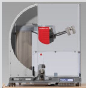
Fig. 3: HIT5.5P safety housing is mounted on the right and can be swiveled to the left
