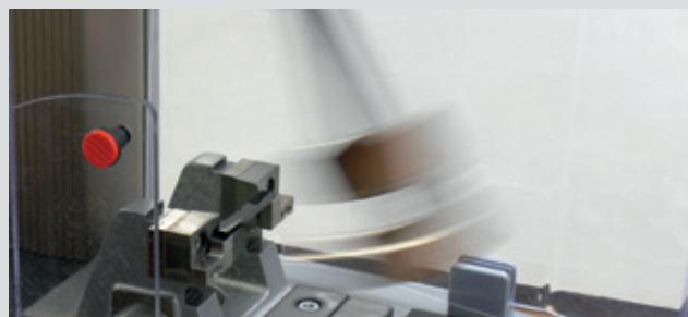
Fig. 3: HIT25P performing a Charpy impact test
