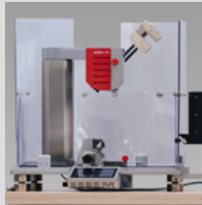
Fig. 1: HIT5P with safety housing fixed on the left and right
