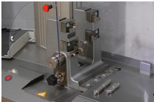
Fig. 1: Charpy fixture with local operator protection, opened
